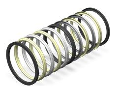
The spring energized seal is a high-performance sealing device engineered with advanced polymers and powered by a corrosion-resistant metal spring. Once seated in the gland, the compressed spring applies consistent force to the sealing surfaces, creating a reliable barrier that prevents the escape of gases or liquids. This resilient design compensates for seal wear, gland misalignment, or eccentricity, ensuring durability.
