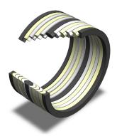
At low pressure, the spring force maintains an effective seal, while at high pressure, the system pressure works in tandem with the spring to deliver an even tighter, more secure seal. SES are expertly machined from PTFE, filled PTFE, and other top-tier polymers, delivering precision and reliability for demanding applications.
